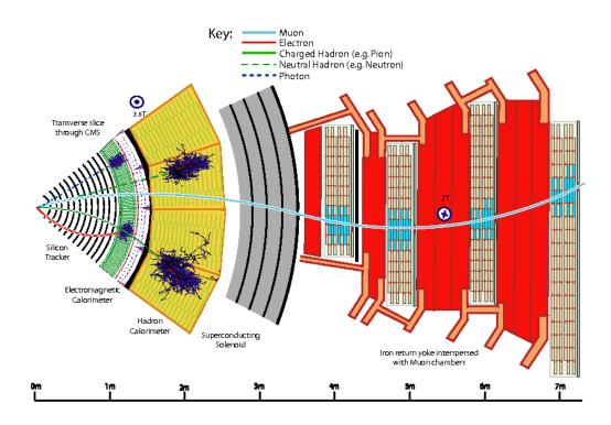
Figure 5.1. Schematic representation of the reconstruction of particles within CMS. An example signature for a muon, electron, charged hadron, neutral hadron, and a photon are shown. The PF algorithm uses the elements from each subdetector (tracks and clusters) to reconstruct and identify the particles, as described in Ref. 31 (from which this figure is taken) and summarized in Section 5.1
